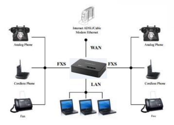
Figure 7: Connecting the HT81X
